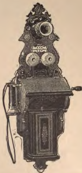
FIG. 9.—Form of Telephone Apparatus, manufactured in Sweden. The magneto-generator and induction coil are enclosed in the box below the call bells; the battery cells, in the cupboard at the base of the backboard. The transmitter is mounted at the top.
